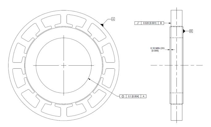
Figure I: Stator Rotor Position Tolerances
